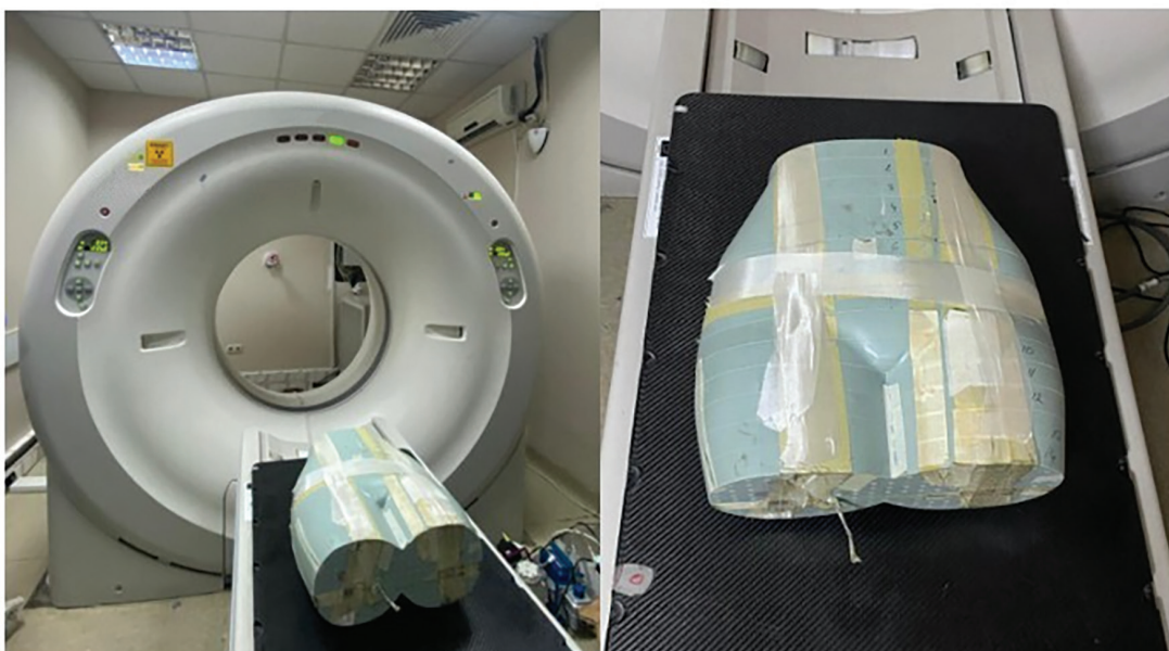
Figure 3. Positioning of the CIRS female pelvic anthropomorphic phantom on the Toshiba Aquilion 64-slice CT scanner. The phantom was placed in the supine position and aligned at the scanner isocenter using the built-in laser positioning system to ensure reproducible imaging geometry during abdominal–pelvic CT acquisitions. CIRS: Computerized Imaging Reference System, CT: Computed tomography
